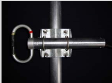
1/4 - wave spacing (1.90 - 2.25 dBd gain) (Offset pattern)
